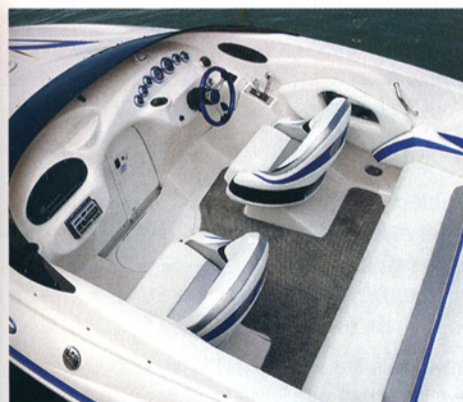
Left: The ZT 244's cockpit included bucket seats with angled bases that served as footrests for those on the rear bench. Right: Checkmate installed a grab handle and a telescoping ladder on the port side of the molded swim platform.
