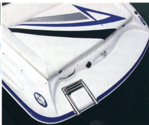
Left: The ZT 244's cockpit included bucket seats with angled bases that served as footrests for those on the rear bench. Right: Checkmate installed a grab handle and a telescoping ladder on the port side of the molded swim platform.
